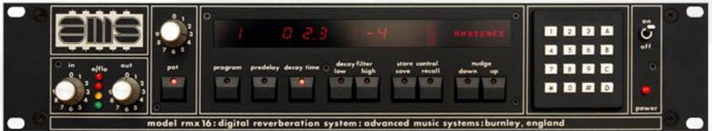
The AMS RMX16 was the world's first microprocessor-controlled, full-bandwidth digital reverberator and characterized an enormous number of seminal recordings from the 1980s onwards. Its designer's love for music and experience in the aerospace industry meant it was way ahead of its time on release.
