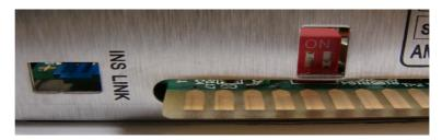
Shown above, the 1073LB EQ switch block set to Standalone mode. All modules are set to this mode when they leave the factory - Switch 1 (left) On, switch 2 (right) Off.
