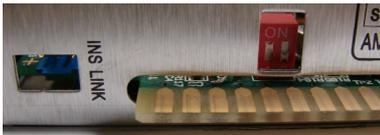
This is used when a 1073LB Mic Pre module uses an adjacent AMS Neve module as a true audio insert across it (for example, the 1073LB EQ) and both modules are set to work in Insert mode (see next page).
