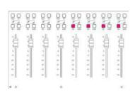
A highlighted/selected track in Logic Pro will also be shown in the Genesys DAW software screen in the top-right corner in *red LCD type font*, 01, 02... 48. The fader SEL button will also flash to indicate the selected track.
