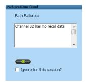
If there is a problem with any of the modules (for example, if one has been removed for repair and there is a gap in the console), a screen will tell you that no Recall data is available for that specific channel strip.
