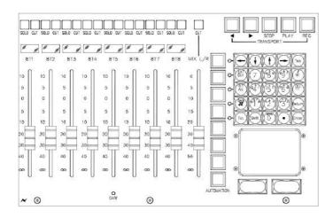
The 8T faders (Master faders) can either control the **8T** fader levels or a block of 8 DAW faders (the red led underneath the faders will light when DAW control has been established).
