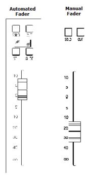
Each fader has a range of  $-\infty$  to +10dB, with it's own **CUT** and **SOLO** button.
