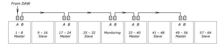
There are a pair of FireWire ports on each Master card and Monitor card labelled  ${\bf A}$  and  ${\bf B}$ .
