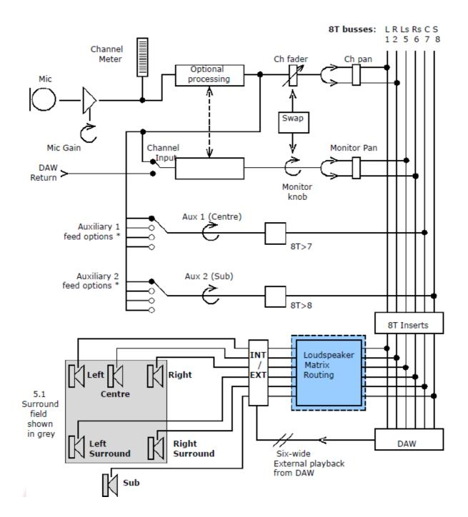
• The Auxiliaries can be fed from either the Channel or Monitor, either Pre- or Post- fader.
