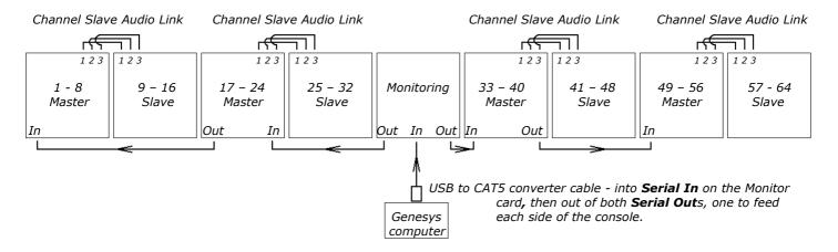
The cards in positions 1-8, 17-24, 33-40 and 49-56 are AD/DA Master cards, each of them connected to their Slave cards by  $3 \times CAT5$  connectors: Serial 1 on the Master connects to Serial 1 on the Slave and so on.
