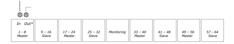
The Wordclock Sync can only be accepted by the left-hand most Master card (or the Monitor card if this is left-most) using the **WCLK IN** BNC connector.
