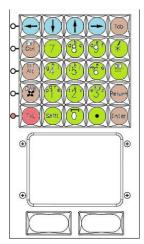
The all-in-one alphanumeric keypad is used for entering filenames on screen when in the Filing screen.
