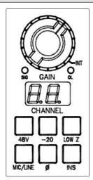
Each channel can be controlled from the front panel, from a remote Mac or PC, or via Pro Tools using the optional remote control software.
