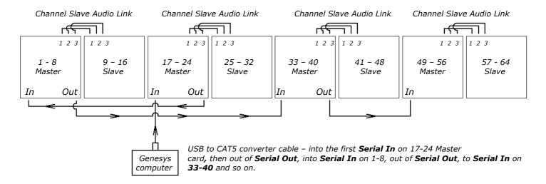
On a system without a Monitor card, the comms goes from the Genesys computers into the 17-24 Master card, then this signal goes to 1-8, 33-40 and finally 49-56.
