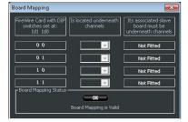
The screen only shows those cards that have been detected on boot-up, so for example, on a 64-fader system that only has 3 Master and 3 Slave cards, only the first three rows on screen will be available for mapping, as shown left.
