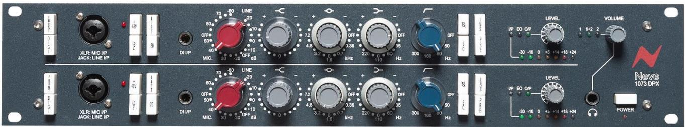
**POWER:** Switches the unit on or off. The adjacent LED lights when the unit is ON
