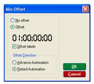
This is used to offset the automation system from the incoming timecode.
