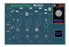
When Recall finds a control that does not match the currently loaded Store, the scan will stop and Recall will display the section(s) and the controls which do not match. The Channel Solo key will also illuminate. For example, on the left is shown the **Monitor Section**.
