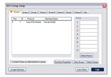
Group Setup is used to setup groups of machines and configure individual machines.
