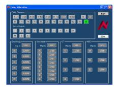
The **Fader Allocation** screen allows you to map any of the large or small faders to control stem inputs and outputs, 2T mixers and the Music, Effects and Dialogue faders (plus the Utility fader, where fitted).
