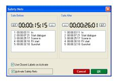
Allows you set up an In and an Out point on the timeline so that automation on either side of these two points is protected against further changes.
