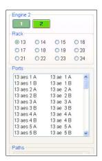
I/O Patch now contains buttons for selecting the display of madi ports relating to a particular engine.
