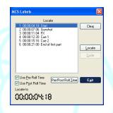
The focus of the MCS Labels dialogue will change to the **Locate To** time which will show the timecode of the selected Label (or zero if no Label has been selected).
