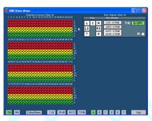
The **Colour Groups/Colour Stems** button swaps between showing all stem members in the same colour but a different colour for each stem (screen above), and colour coding each part of the stem, so LCR is red, LS/RS is yellow and 7/8 is green uniformly for each stem (screen left).
