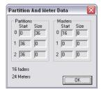
The Partition and Meter Data dialogue box will be displayed. This shows the size of each partition, the size and position of each Master section, the size of the desk and the number of meters.
