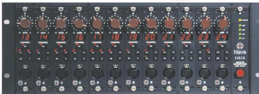
The 1081R is a front end microphone pre-amplifier, using amp circuitry similar to the classic '1081' design of the early 1970s. The PC and Pro Tools options offer the added benefit of a recall system for all settings.
