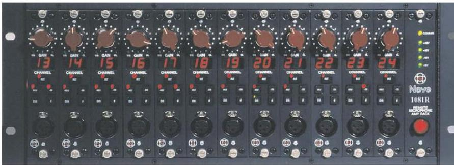
Twelve modules can be fitted into the 4U rack housing.
