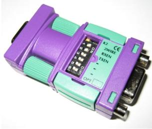
Most PC's are fitted with RS232 interfaces as standard and will therefore need to use the RS232 to RS485 converter (such as ones manufactured by K2 systems, shown left). This is a female-to-female 9-pin converter that goes between the rack and the PC.
