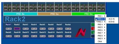
When all parameters have been set correctly, the colour-coded mapping will be displayed on the main **Mic** programme page.
