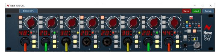
The 1073OPX proprietary Remote-control software application can be run on Mac or PC and allows users to access and operate the 1073OPX control features remotely. The unit's front panel controls including gain level, Input selection, phantom power, etc can be controlled remotely from any connected computer.
