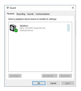
Once installed, the 1073OPX will appear in your PC's available audio devices and the AMS NEVE USB audio device control panel application can now be accessed. This application allows users to view the selected sample rate, Bit Depth, buffer size, I/O and release and serial number information.
