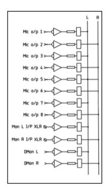
The Monitor output XLR connectors at the rear of the unit follow the front **HP LEVEL** monitor signal selection. This function gives users the ability to use the unit as a 4x stereo input analogue summing mixer. Users can pass audio signals through the 1073 line-level preamplifiers, combining them into the monitor path through the Left and Right Monitor output XLRs on the rear of the unit. This stereo signal can then be fed into the DAW and recorded back as a summed stereo track.
