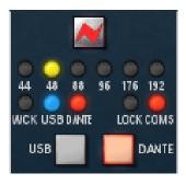
This mode enables the 1073OPX to function as a Dante networked audio device which can be accessed by the connected Dante network.
