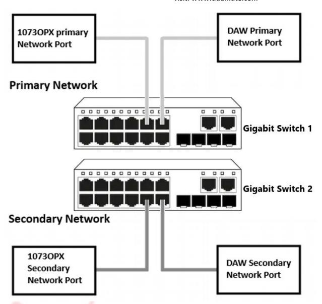
All D<mark>ante connections should</mark> be made using CAT5e or CAT6 ethernet cable and connections must be made by using gigabit switches.
