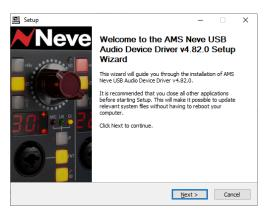
Download the AMS Neve USB Audio Device Driver from www.AMS-Neve.com >1073OPXproductpage >supporting documentation for your PC, run the application and follow the on-screen instructions. Before installing, please ensure that the USB cable is disconnected from the unit
