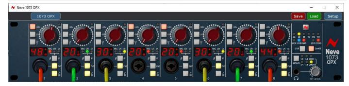
When communication is synchronised between the 1073OPX and the GUI, the **COMMS** light will illuminate red. Two-way control between the plugin and the unit front panel controls is now possible. Changes made on the front panel of the unit will be reflected in the plugin. Similarly, changes made on the plugin will be reflected on the unit front panel controls.
