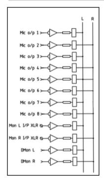
The 1073OPX monitor path can be fed from a combination of preamplifier output and monitor input signal sources. This enables latency free monitoring of preamp signals, allowing operators to record overdubs by listening to the input source directly pre-DAW. Users can blend the mic, line or DI preamplifier signals directly with the monitor or digital monitor signal for quick latency-free monitoring.
