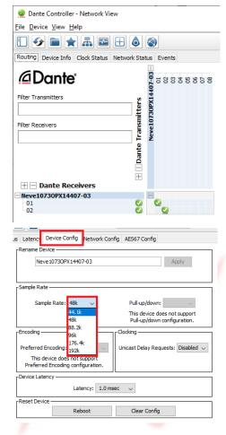
The Dante controller software allows users to route any of the 1073OPX audio paths to any available network audio device via the simple routing matrix on the main screen. The 1073OPX 8 preamplifier outputs will be shown on the Dante Transmitters tab and the 2 digital **DMON** inputs will appear on the Receivers tab.
