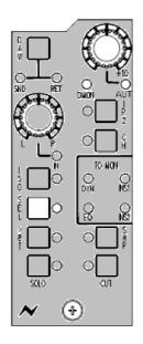
➤ You can send all of the Channel Inputs (or MON Returns) to the Left and Right of the Main Mix buss by clicking the MIX L/R after selecting the CHANNELS tab (or MONITOR tab) button (see image to the left).
