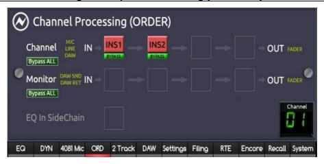
You can manually control the channel processing order using the ORD button on the Channels to set/show the order processing of the EQ/DYN/INS1/INS2 (elements).
