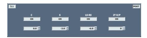
There are individual On/Off controls and +/-10dB of Trim for each of the  $\bf C$ ,  $\bf S$  and  $\bf LS/RS$  contributions to the 2T Output, plus a global On/Off and level control ranging from 0dB to  $\infty$  for the 2T Output.
