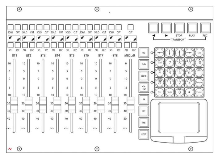
The 8T faders (Master faders) can either control the **8T** fader levels or a block of 8 DAW faders (the red LED underneath the faders will light when DAW control has been enabled).
