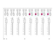
A highlighted/selected track in the DAW will also be shown in the Genesys DAW software screen in the top-right corner in *red LCD type font*, 01, 02... 48. The fader SEL button will also flash to indicate the selected track.
