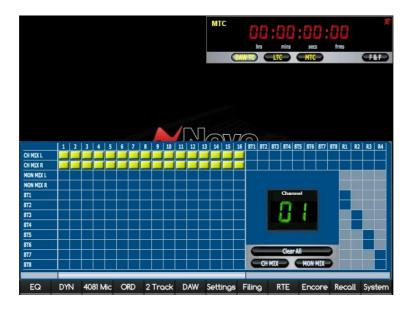
This screen is a graphic representation of the internal routing of the console and is shown whenever the **RTE SEL** button is pressed (depending on how this Preference is set up in the **Settings** screen).
