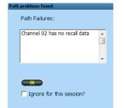
If there is a problem with any of the modules (for example, if one has been removed for repair and there is a gap in the console), a screen will tell you that no Recall data is available for that specific channel strip.
