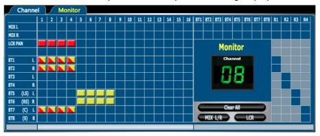
In the Routing Screen, there is a tickbox that enables the LCR Pan routing functionality.
