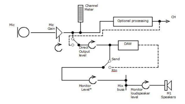
• The Monitor level is set using the Monitor knob on the lower section of the Channel strip. If you wish this control to be on the fader instead, press the **SWP** button on the Master SEL panel to swap all the faders over, or use the local **SWP** button to swap individual faders.
