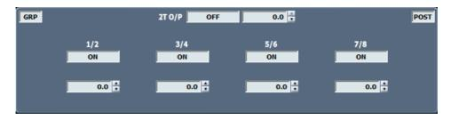
This screen configures the automatically-created 2 Track mix. The screen that opens depends on how the 2T has been set up to operate, either in **Group Mode** (shown above) or **5.1 Mode**.
