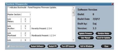
The list of Panels on the left side of the screen shows not only which panels have been detected (as indicated by a 'Y' being shown against it), but also which internal communications link each panel is communicating on.
