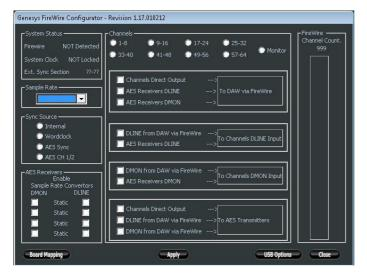
The Configurator allows the routing of the digital audio signals in blocks of 8 channels (1-8, 9-16 etc and not on a channel-by-channel basis).
