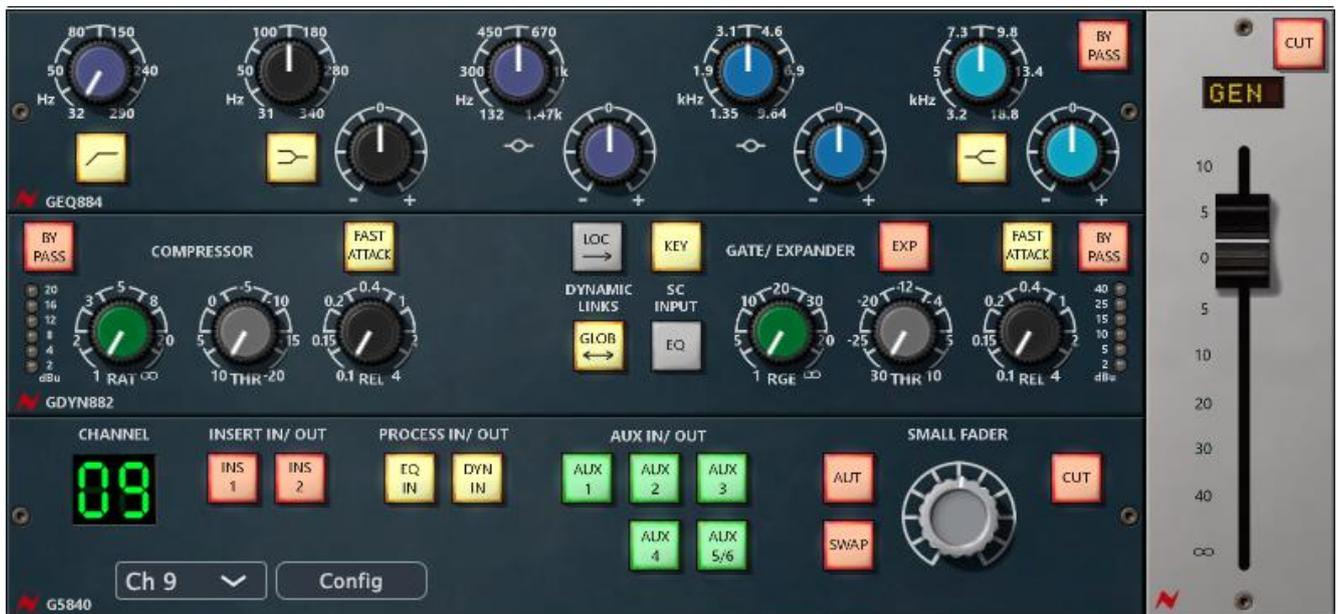
GenesysControl Plugin displaying 88REQ, VCA Dynamics and Channel Strip control
