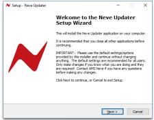
The Neve firmware update software can be found at www.AMS-Neve.com >1073OPXproductpage >supporting documentation. The software program is used to check your unit's firmware is up to date and perform the necessary updates if required. The windows application is 32-bit software supported by windows 10. The MAC 64-bit software supports OSX 10.14/10.15 only.
