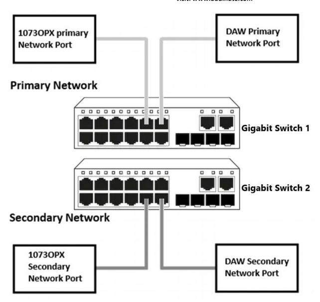
All Dante connections should be made using CAT5e or CAT6 ethernet cable and connections must be made by using gigabit switches.
