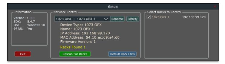
Once the units IP address has been assigned, the remote software will scan for connected devices and automatically connect. If a unit is not found, or if several 1073OPX units are connected, click the **SETUP** button in the plugin software window and follow the steps on the following pages.
