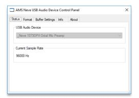
The 1073OPX will now function as an ASIO/core audio device and is compatible with sample rates up to 192kHz and bit depths of 16/24Bit.
