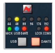
Depending on the Digital option card installed, there will be either Wordclock Input and Output connections (USB/Dante card), or a Wordclock Input connection only (USB/ADAT card).
