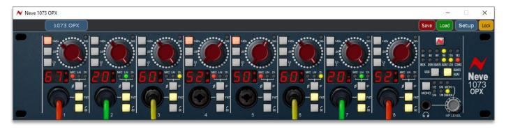
The 1073OPX proprietary Remote-control software application can be run on Mac or PC and allows users to access and operate the 1073OPX control features remotely. The unit's front panel controls including gain level, Input selection, phantom power, etc can be controlled remotely from any connected computer.
