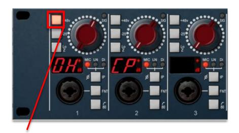
To view the manual address menu and set a manual IP Address, press the Preamplifier Channel 1 +48v button.
