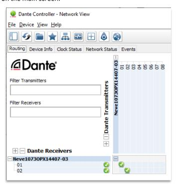
This window uses a matrix with horizontal and vertical tabs to connect units together, active connections are called subscriptions.
