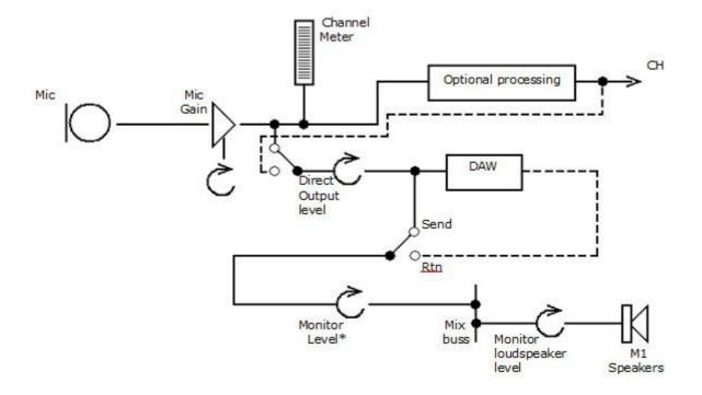
• The Monitor level is set using the Monitor knob on the lower section of the Channel strip. If you wish this control to be on the fader instead, press the **SWP** button on the Master SEL panel to swap all the faders over, or use the local **SWP** button to swap individual faders.
