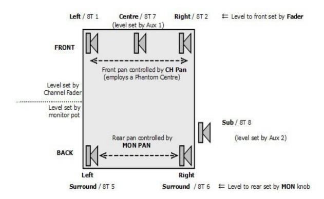
Using the Fader and Monitor Pot (and the associated pan controls on each fader strip), a signal can be sent to any point within the surround field.
