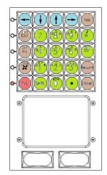
The all-in-one alphanumeric keypad is used for entering filenames on screen when in the Filing screen.
