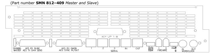
This cassette provides 8 channels with AD/DA converters. Depending on the digital channel requirements, a Master or Master and Slave card can be installed in groups or individually.
