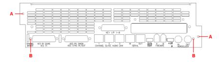
► Unscrew the blanking plate that is fitted to the lower half of the plate, removing the two screws labelled 'B' above.
