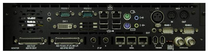
This computer cassette has the optional Monitor Section Digital Board fitted. The connectors on the bottom row are for this option.
