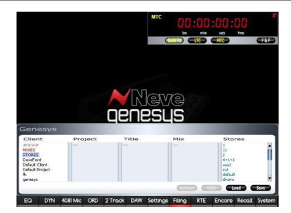
Provides the facility to **Save** and **Load** Snapshot and Recall files, either to/from the local hard drive or local USB port.
