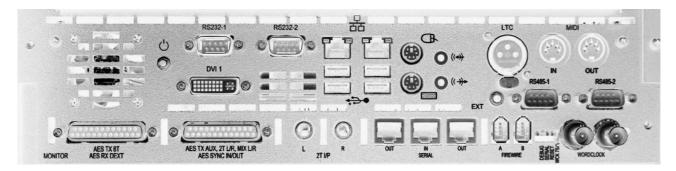
This single card (regardless of console size), enables the **Main Mix**, **2T**, **8T** and **Auxiliary Sends** to be sent from the desk digitally, as well as accepting a **5.1 Digital Surround External** into the monitoring system to be sent to the loudspeakers.
