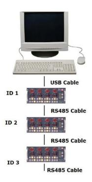
It is possible to 'daisy-chain' multiple units together so they are controlled via USB on a Mac or PC.
