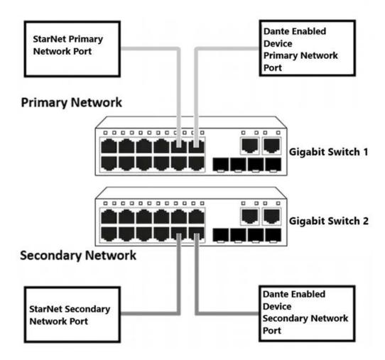
The StarNet ADA16 has both a **PRIMARY** Dante network port and a redundant **SECONDARY** Dante network port.
